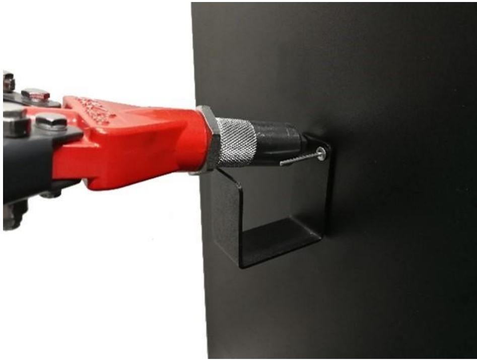
Figure 27. Hook riveting method
