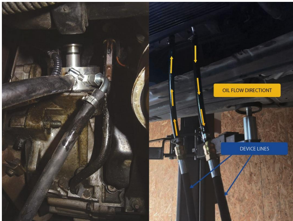
Figure 6. Method of connecting the device adapters to the transmission. On the right: Connection to the ATF line of the transmission cooling system. On the left: In this case, in the AW55-50 transmission, the round heat exchanger was replaced with a special adapter (with a gasket and spacers).
