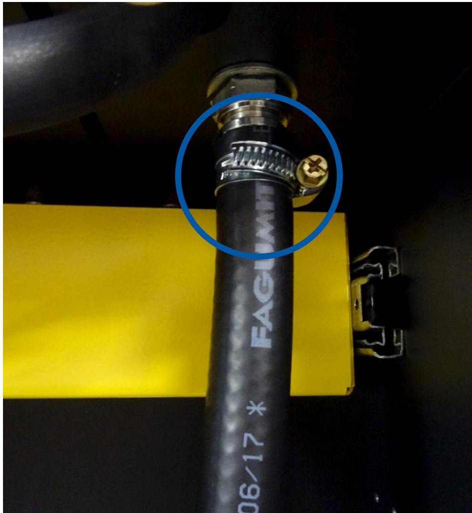
Figure 25. Clamp used for adjusting the length of the suction hose
